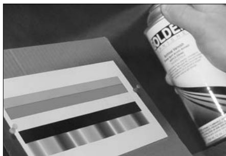
Three ways to seal a print include spraying with GOLDEN Archival Varnish, brushing with GOLDEN MSA Varnish or applying MSA Gel with a squeegee. These Mineral Spirit Acrylic-based products should not distort water sensitive prints.
