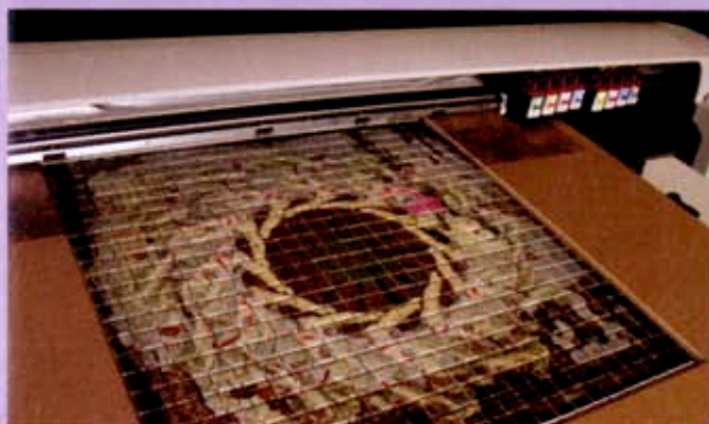
A Fome-Cor® lightweight, laminated, board tray holds pre-coated ceramic tiles as they're printed on an Encad 880 flexible-media printer.
