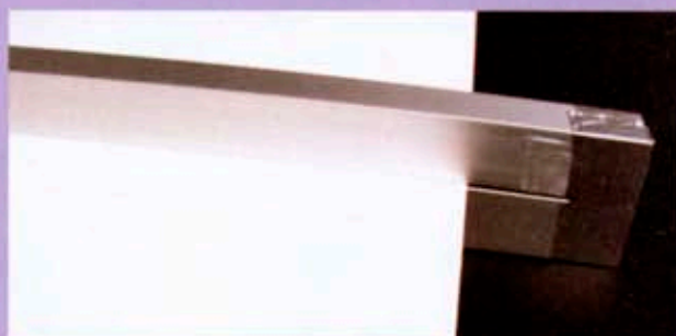
Use a slot ruler to avoid head strikes. Place coins or other objects equal to your printer's clearance at the ends of two square, aluminum tubes, and secure them with duct tape. Slide your substrate through to check for high spots before printing. Printers that accept mat board have 1.5mm clearance, the thickness of a new penny.
