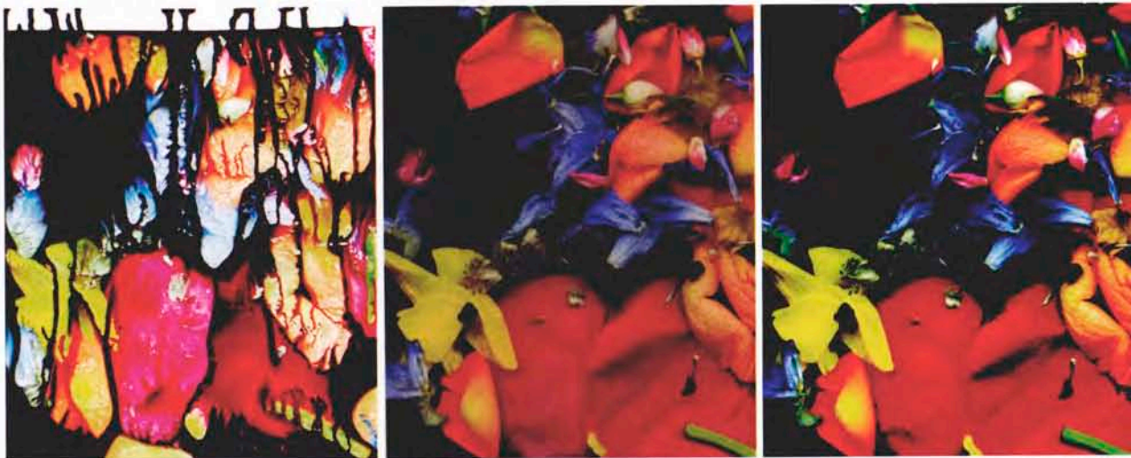
At left, printing on untreated, nonabsorbent material like this plastic sheet causes the ink to run. Middle, untreated newsprint is too absorbent, producing a soft, dull print. At right, commercially treated fine-art paper gives this print its sharper, brighter image.
